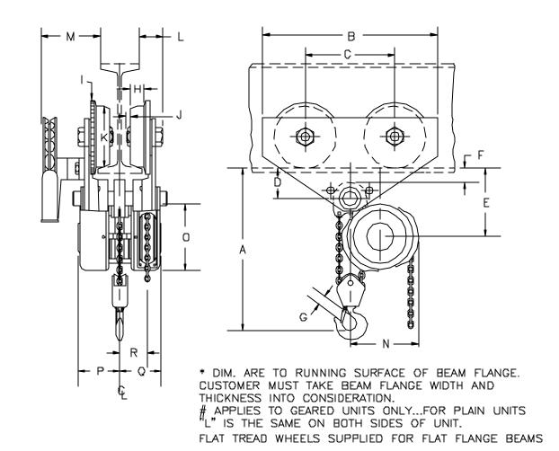
THIS UNIT IS ADJUSTABLE FROM 4" - 7 1/8" FLANGE WIDTH FLAT OR TAPER FLANGE MUST BE SPECIFIED AT TIME OF ORDER
