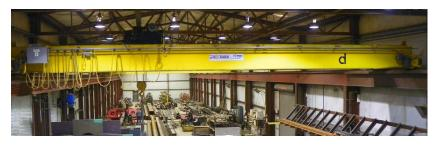
Applications for moderately rated, or Class C, cranes, include medium-grade machine shops, paper mill machine rooms, and other mid-grade manufacturing set-ups. These tools can handle five to ten lifts an hour, with an average load weighing in around 50% of their rated capacity, averaging 15 feet, not over 50% of the lift at rated capacity.
