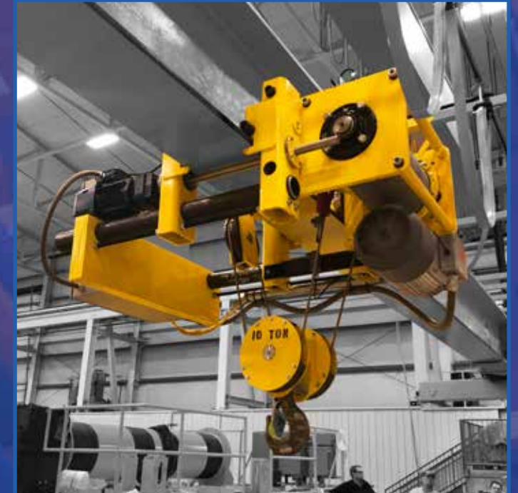
ACECO Bridge Crane utilizing ACECO NorHoist
