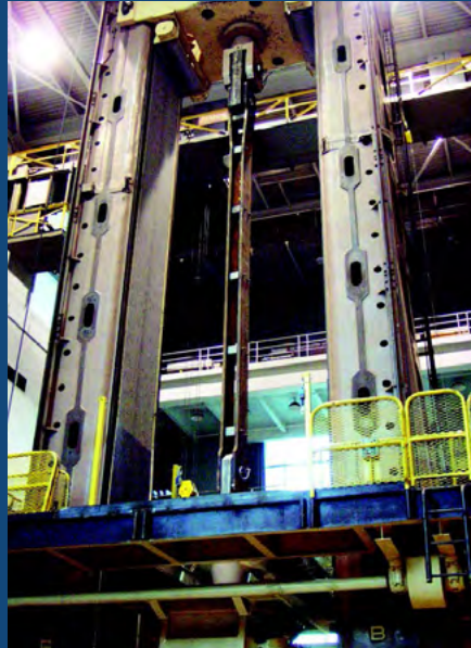
CASK LIFTING YOKE EXTENSION SHOWN DURING 390 TON PROOF TEST
