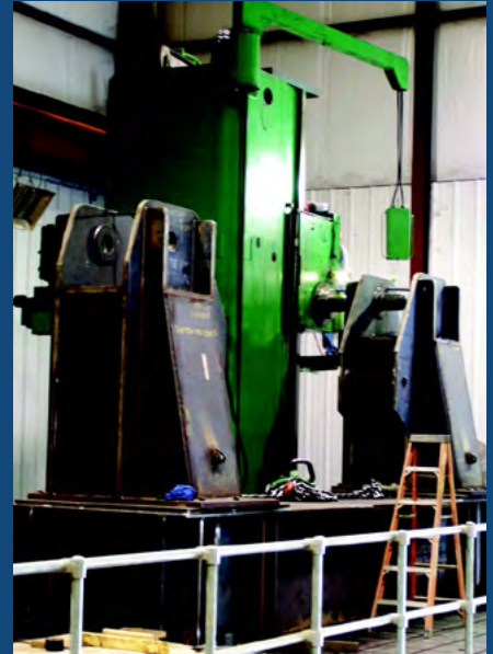
7" GIDDING AND LEWIS FLOOR TYPE HORIZONTAL BORING MILL WITH 30' HORIZONTAL & 13' VERTICAL TRAVEL SUPPORTED WITH 30 TON OVERHEAD CRANE
