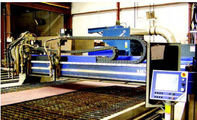
STATE-OF-THE-ART PLASMA AND OXY-FUEL CUTTING MACHINE FEATURING 10' X 42' CUTTING TABLE
