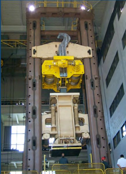
475 TON PROOF LOAD TEST OF SAFLIFT™ SPECIAL LIFTING DEVICE FOR DRY STORAGE CASK SEISMIC STABILITY
