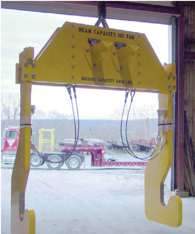
105 TON CASK LIFT BEAM
